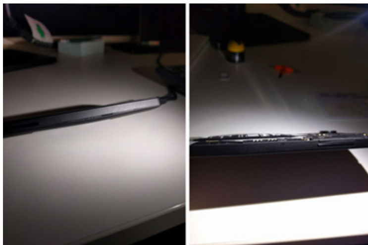
Figure 8.- Battery deformed by the excessive heat generated.
